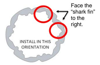
**NOTE:** Proper orientation of the drive plates is *critical* for optimal clutch performance. If you install them backwards, the clutch will still function but will lack proper modulation performance.
