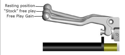
Optimal Free Play Gain yields 1/8" (3mm) of clutch lever movement, measured at the end of the lever. This measurement at the lever correlates to achieving the ideal installed gap.
