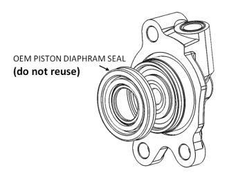
**NOTE:** The Rekluse slave cylinder comes preassembled in the kit. If the parts are separated, assemble them in the following order: Rekluse slave cylinder, supplied O-ring, then the supplied paper gasket.
