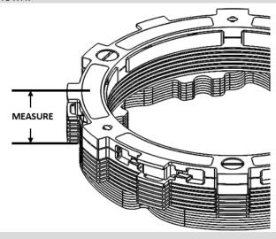
This measurement needs to be 1.343"-1.355" [34.1mm-34.4mm] tall. If it is taller than that, take out 1x .048" [1.2mm] drive plate and replace with 1x .040" [1mm] drive plate and remeasure. Repeat until the desired pack thickness is attained.
