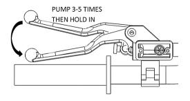
**38.** Using an 8mm wrench, open the bleed port while continuing to hold on the clutch lever at the handlebar. Air and fluid may flow from the bleed tube. Tighten the bleed port when pressure is lost.
