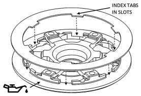
**19.** Install the pressure plate subassembly.
