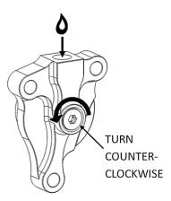
f. Compress the piston until it bottoms out. Repeat steps  $\mathbf{c}_{\cdot} - \mathbf{f}_{\cdot}$  until there is no longer air escaping from the top port when the piston is compressed.
