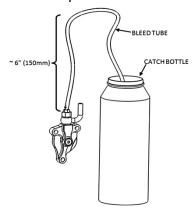
**37.** Pump the clutch lever 3-5 times then hold it against the bar/grip. Top off the fluid.
