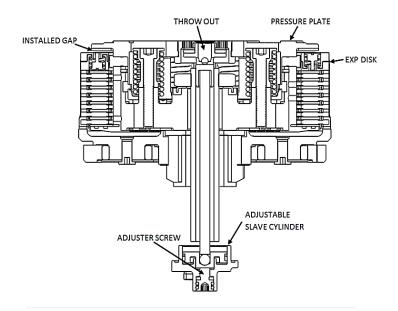
**42.** Using the long end of a 4mm Allen key, turn the adjuster screw clockwise until it stops under moderate pressure. You are trying to feel for the point at which the throw-out will start to lift the pressure plate. This is the "starting point."
