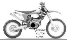
**NOTE**: Take note of each OEM clutch cover bolts specific location as length can vary between them. Failure to replace these bolts in the proper location after clutch installation can result in damage to your motorcycle.
