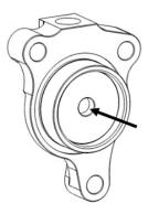
c. Pour clutch fluid into the slave cylinder port.
