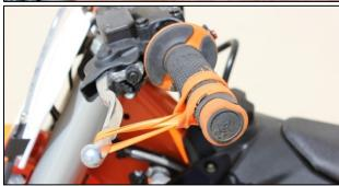
With the bike at idle in neutral, **quickly** blip (rev) the engine to at least 5,000 RPM and let it return to idle. **The clutch lever should move in about 1/8" (3mm) toward the handlebar as you rev the engine.** Turn the Slave Cylinder adjuster screw clockwise 1 tick at a time until optimal clutch lever movement (i.e. Free Play Gain) is achieved.
